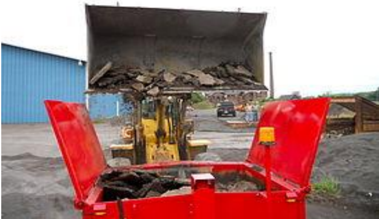
Fig3.Chunks of Reclaimed Asphalt Pavement (RAP) are deposited for recycling.
