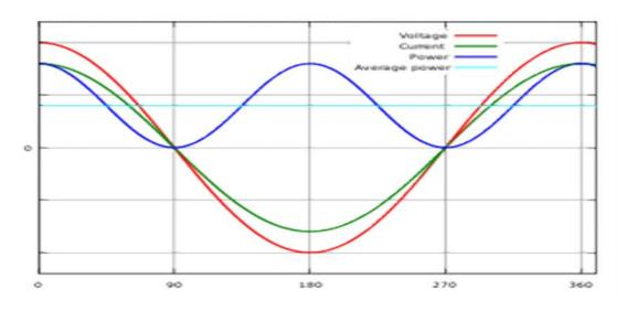
Instantaneous and average power calculated from AC voltage and current with a unity power factor ( $\varphi = 0$ ,  $\cos \varphi = 1$ ). Since the blue line is above the axis, all power is real power consumed by the load.
