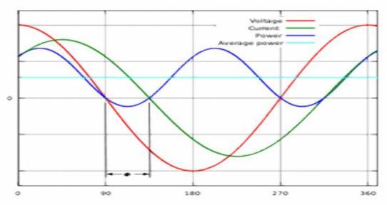
Instantaneous and average power calculated from AC voltage and current with a lagging power factor ( $\varphi = 45$ ,  $\cos \varphi = 0.71$ ). The blue line shows some of the power is returned to the grid during the part of the cycle labeled
