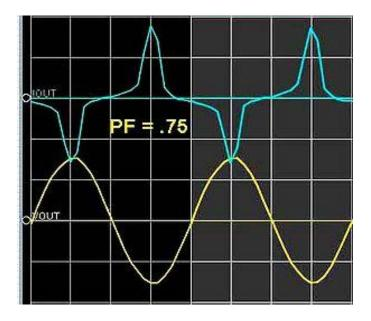
Sinusoidal voltage and non-sinusoidal current give a distortion power factor of 0.75 for this computer power supply load.
