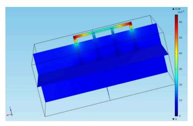
Simulation of multiple grounding in one layer soil
