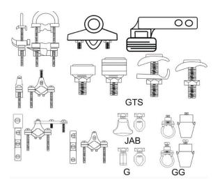
Connectors for earthing installation are a means of communication between the various components of the earthing and lightning protection installations (earthing rods, earthing conductors, current leads, busbars, etc.).
