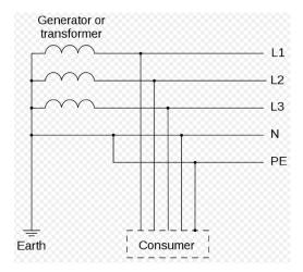
TN-S: separate protective earth (PE) and neutral (N) conductors from transformer to consuming device, which are not connected together at any point after the building distribution point.
