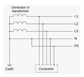
**TN-C-S**: combined PEN conductor from transformer to building distribution point, but separate PE and N conductors in fixed indoor wiring and flexible power cords.
