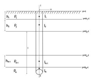
Soil resistance is a major aspect in the design and calculation of an earthing system/grounding installation. Its resistance depends on the efficiency of the removal of unwanted currents to zero potential (ground). The resistance of a geological material depends on several components: the presence of metal ores, the temperature of the geological layer, the presence of archeological or
