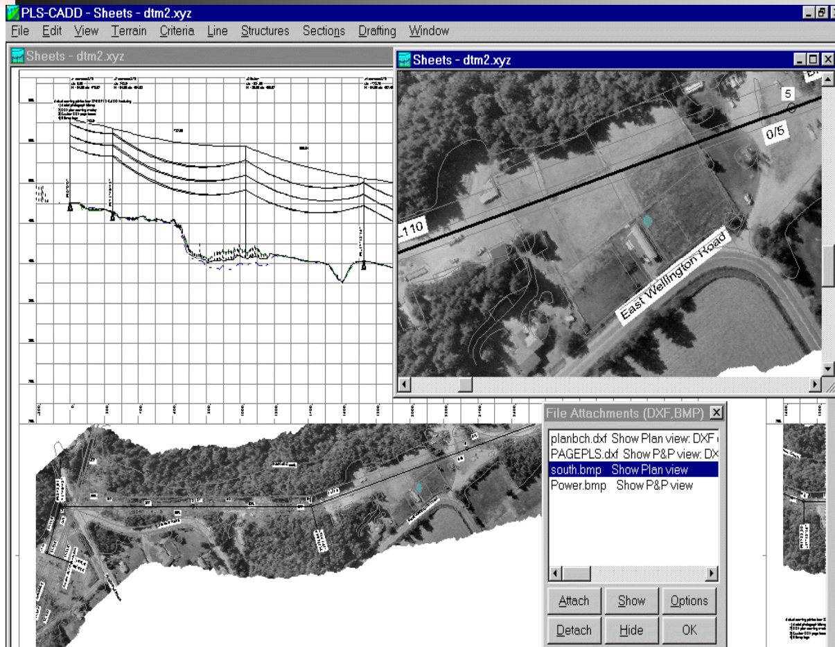
Fig. 1 • PLS-CADD Plan & Profile Sheet With Page Border, Plan Overlay, Logo and Aerial Photo
