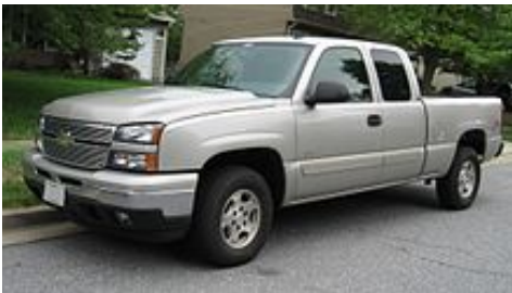
The 2005-06 Chevrolet Silverado Hybrid is a mild hybrid using the electric motor mainly to power the accessories
