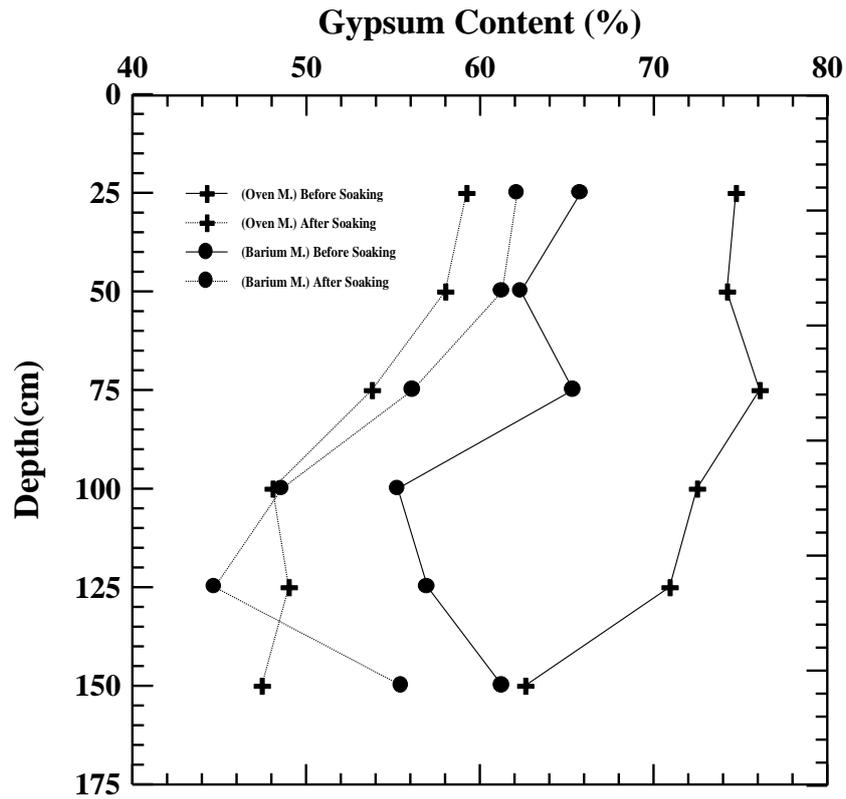
Figure (5.12) Gypsum Content versus Depth by Two Methods
