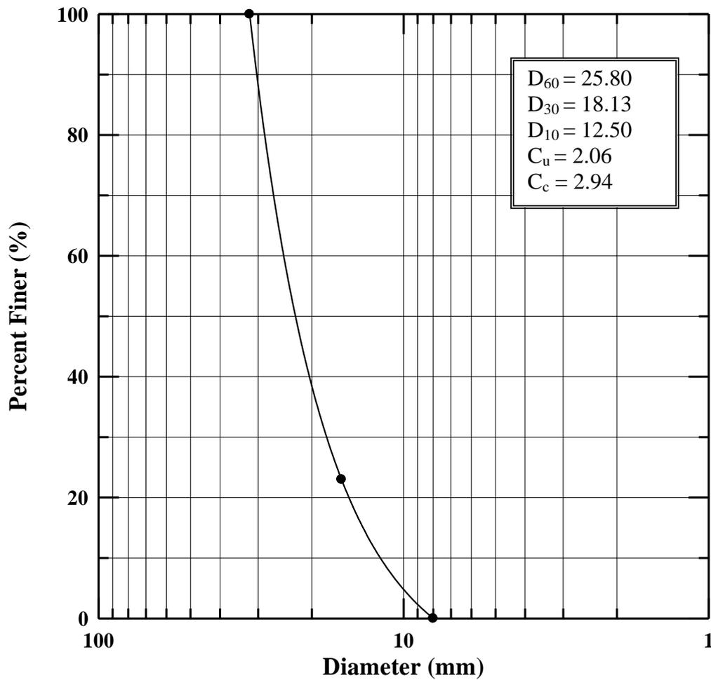
**Figure (4.4) Particle Size Distribution for the Crushed Stone Used**
