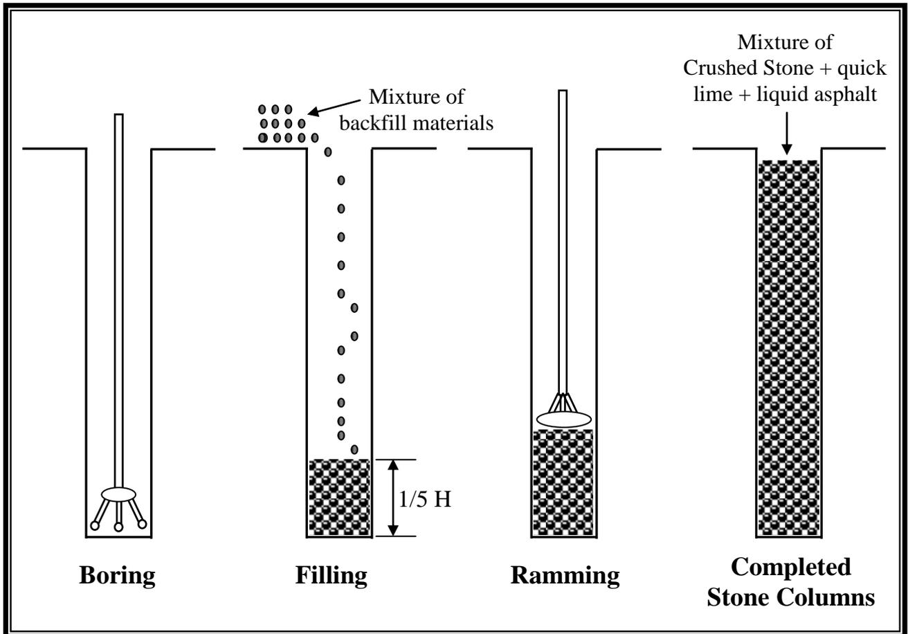
*Figure (4.5) Boring, Backfilling and Ramming Technique*
