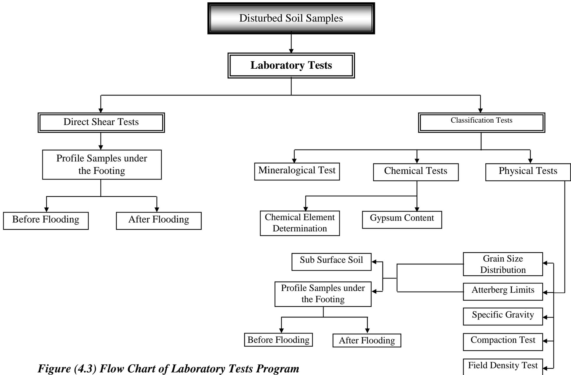
Figure (4.3) Flow Chart of Laboratory Tests Program
