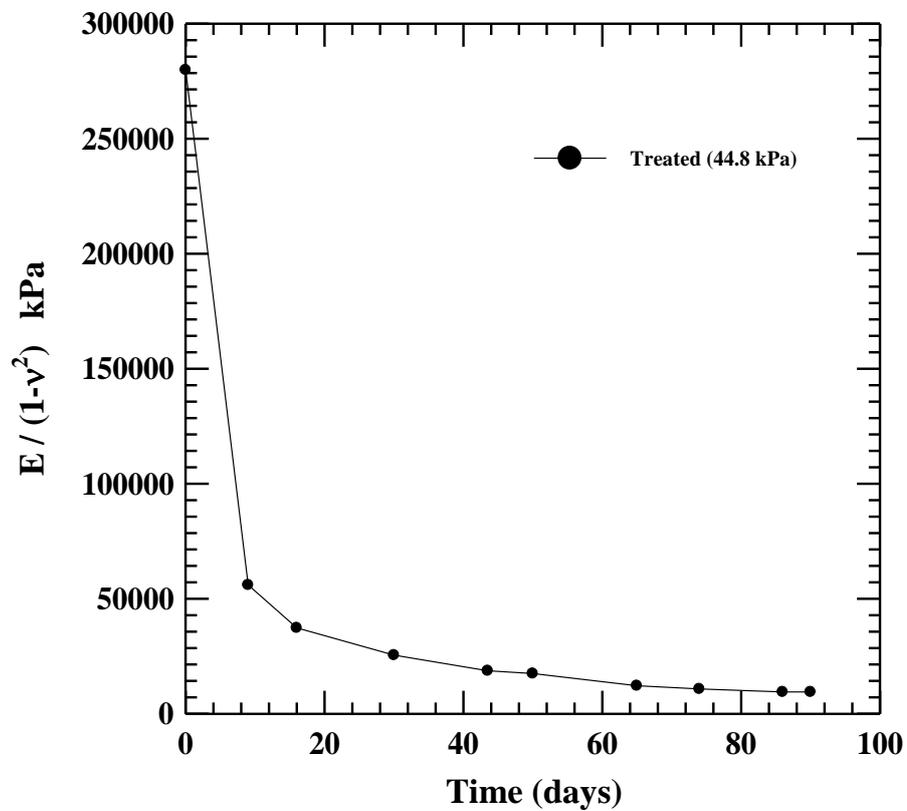
*Figure (5.23)  $E / (1-\nu^2)$  versus Time of Field Test No.4*
