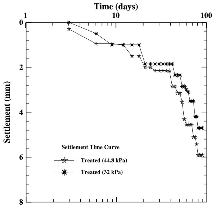
*Figure (5.25) Settlement versus Time (Semi log Scale)
