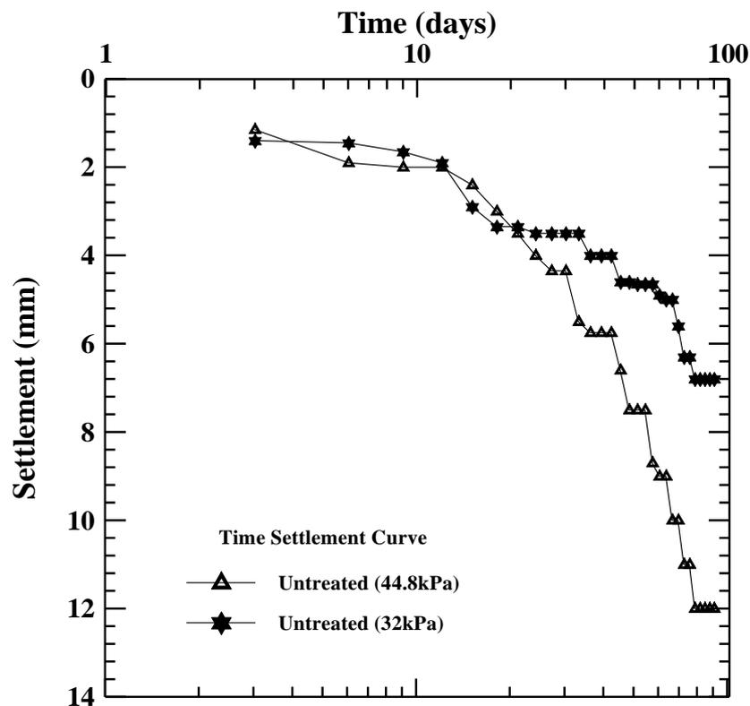
*Figure (5.8) Settlement versus Time (Semi log Scale) (Effect of Applied Stress)*
