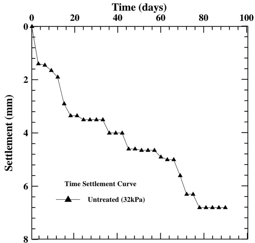
Figure (5.1) Settlement versus Time of Field Test No.1
