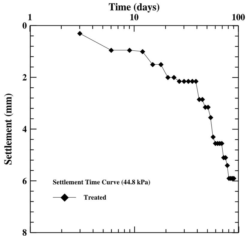
*Figure (5.22) Settlement versus Time (Semi log Scale) of Field Test No.4*
