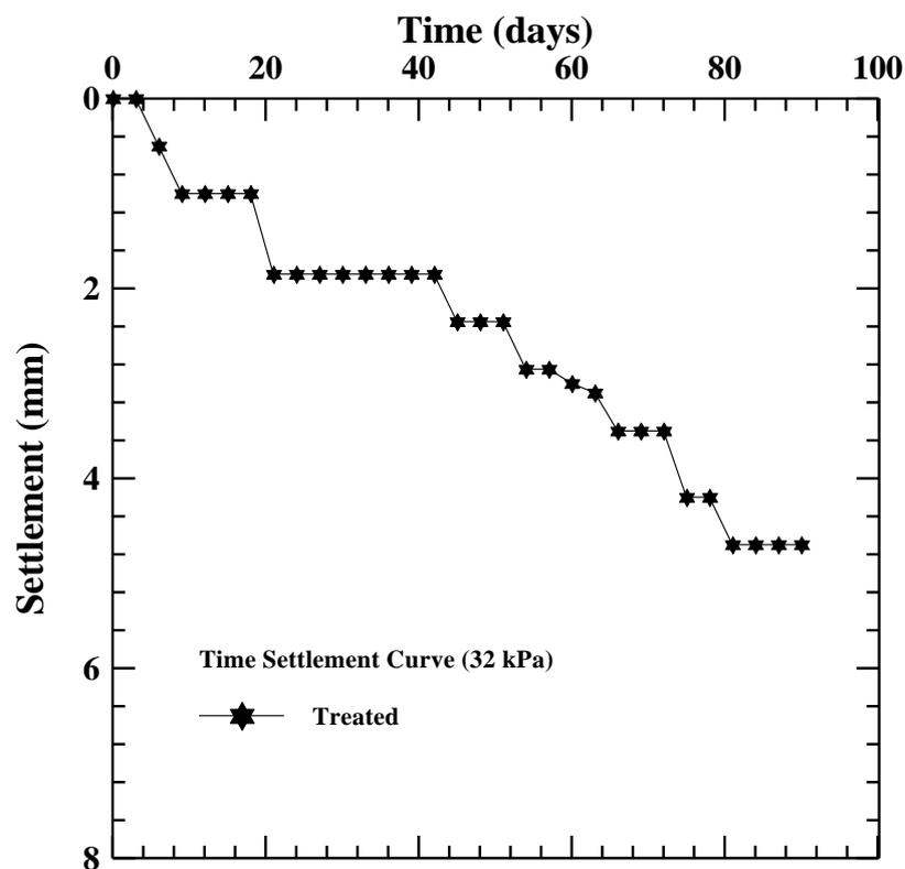
*Figure (5.18) Settlement versus Time of Field Test No.3*
