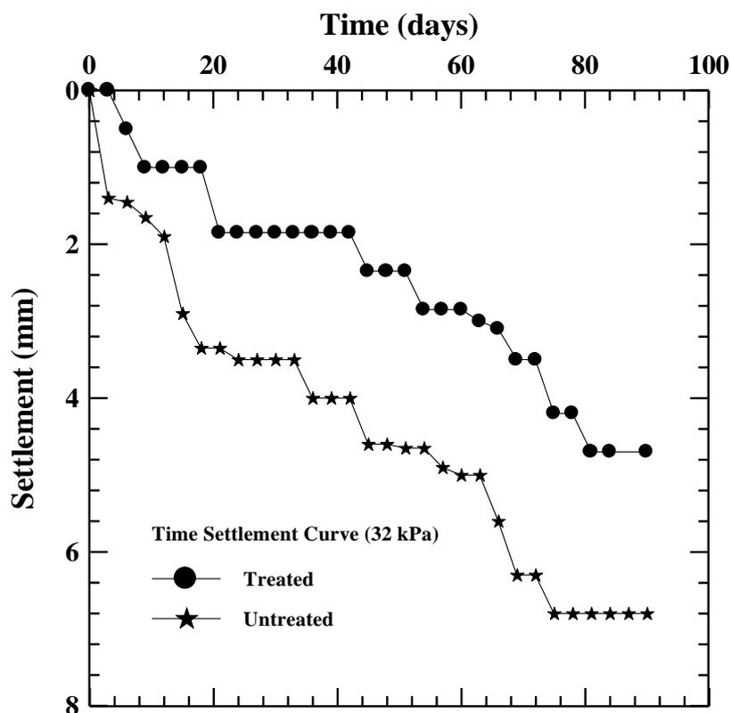
***Figure (5.28) Settlement versus Time (Applied Stress = 32 kPa)***
