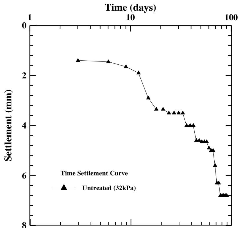
Figure (5.2) Settlement versus Time (Semi log Scale) of Field Test No.1
