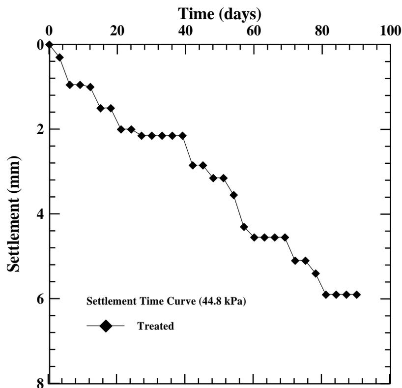
*Figure (5.21) Settlement versus Time of Field Test No.4*
