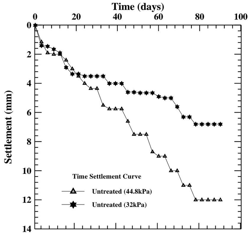
*Figure (5.7) Settlement versus Time (Effect of Applied Stress)*
