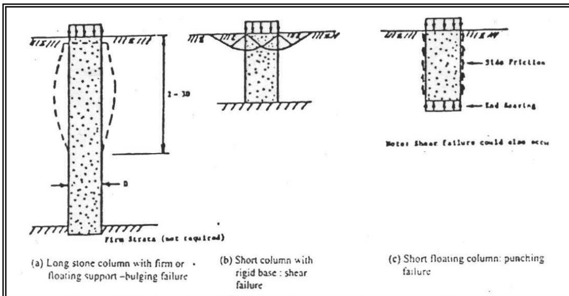
**Figure (3.1) Mode of Failure for a Single Stone Column
