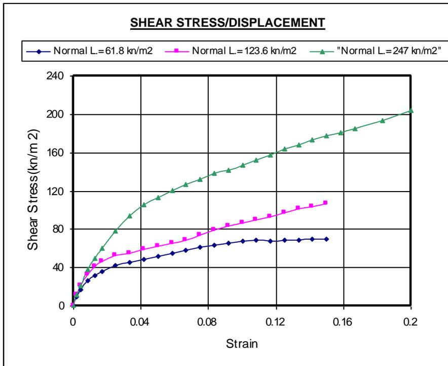
*Results of Direct Shear (Sample 3, After Flooding)*
