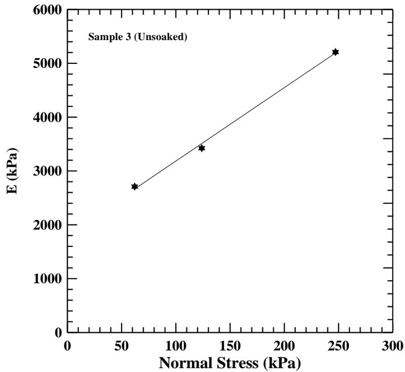
*Results of Modulus of Elasticity (Sample 3, Before Soaking)*
