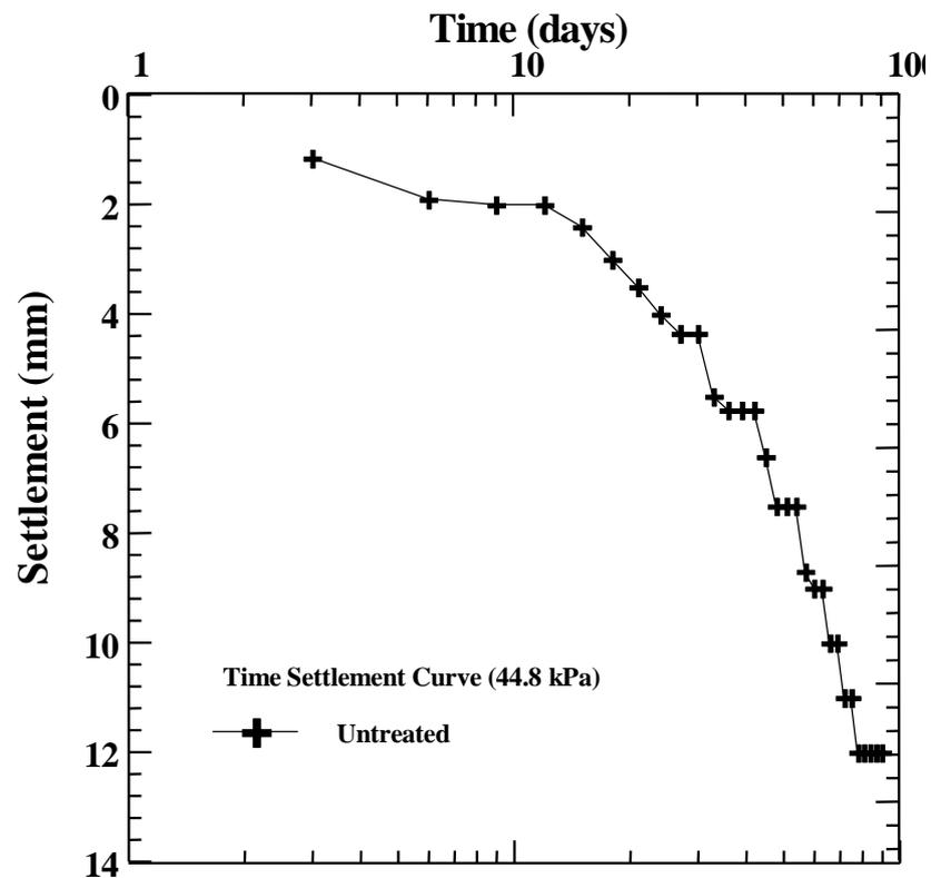
*Figure (5.5) Settlement versus Time (Semi log Scale) of Field Test No.2*
