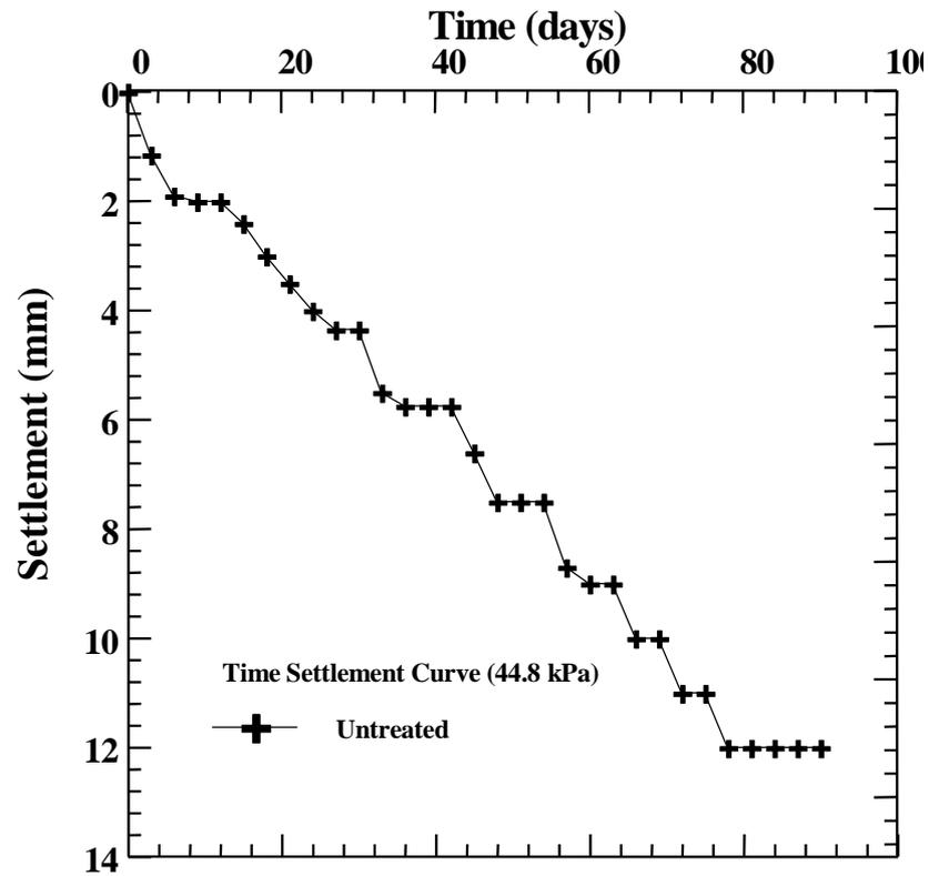
*Figure (5.4) Settlement versus Time of Field Test No.2*
