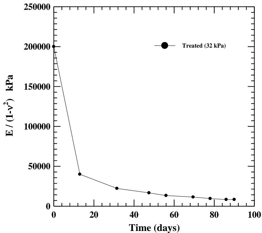
Figure (5.20)  $E / (1-\nu^2)$  versus Time of Field Test No.3
