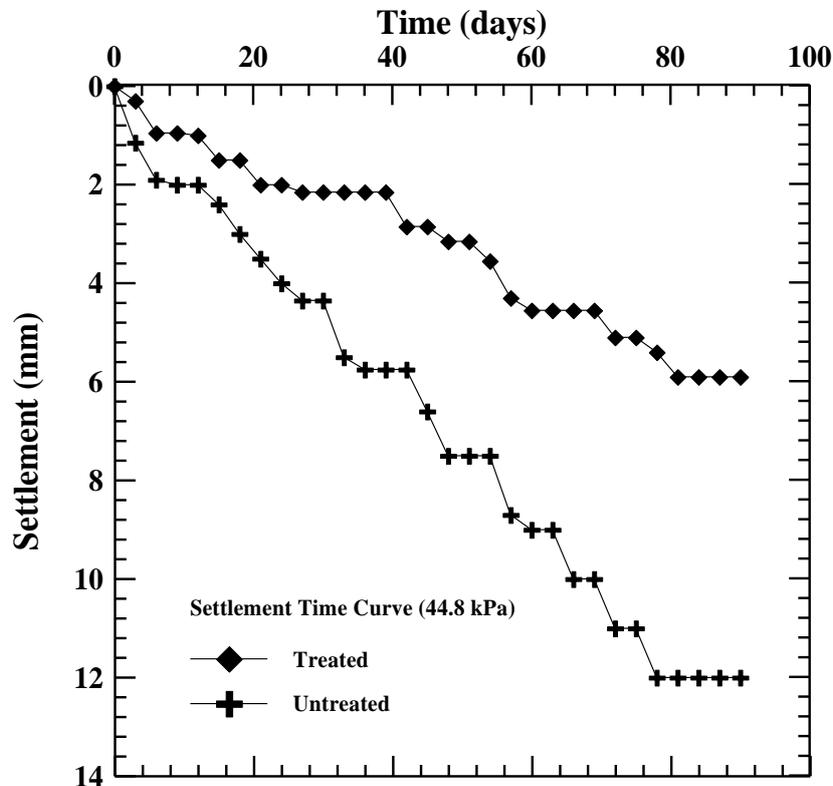
**Figure (5.31) Settlement versus Time (Applied Stress = 44.8kPa)**
