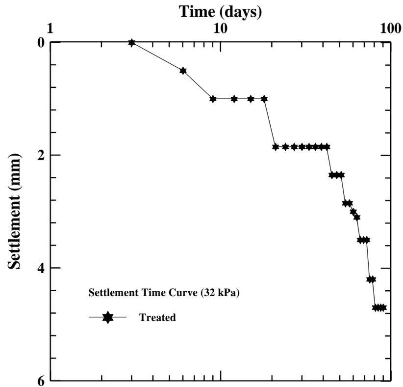
Figure (5.19) Settlement versus Time (Semi log Scale) of Field Test No.3
