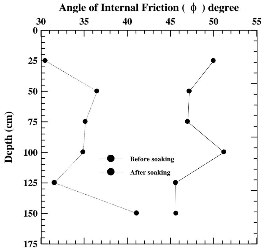
Figure (5.16) Angle of Internal Friction Variation with Depth
