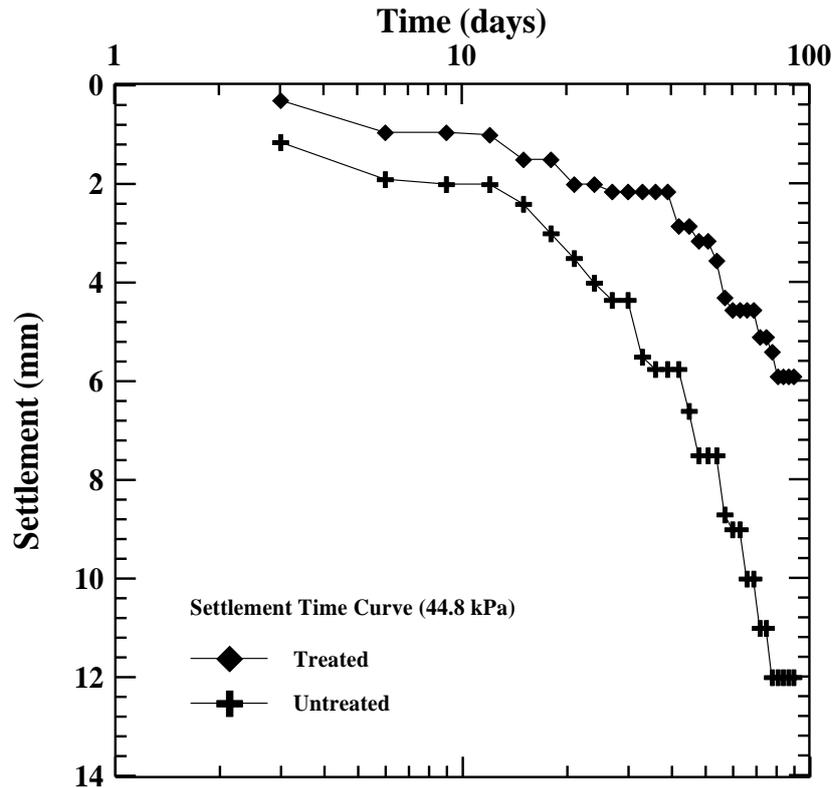
**Figure (5.32) Settlement versus Time (Semi log Scale)
