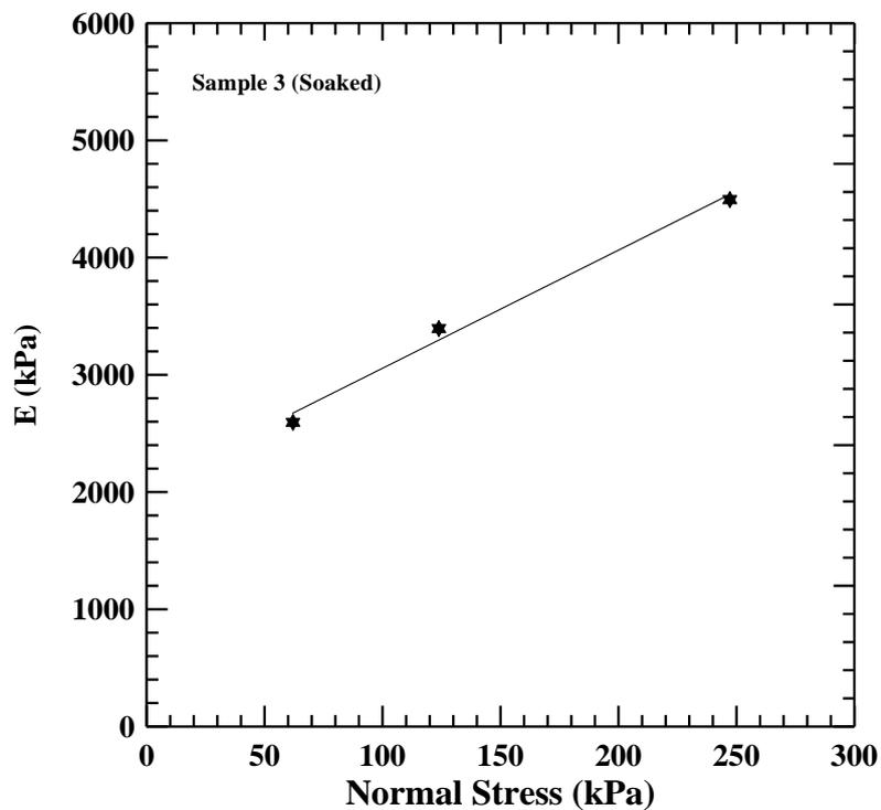
*Results of Modulus of Elasticity (Sample 3, After Soaking)*
