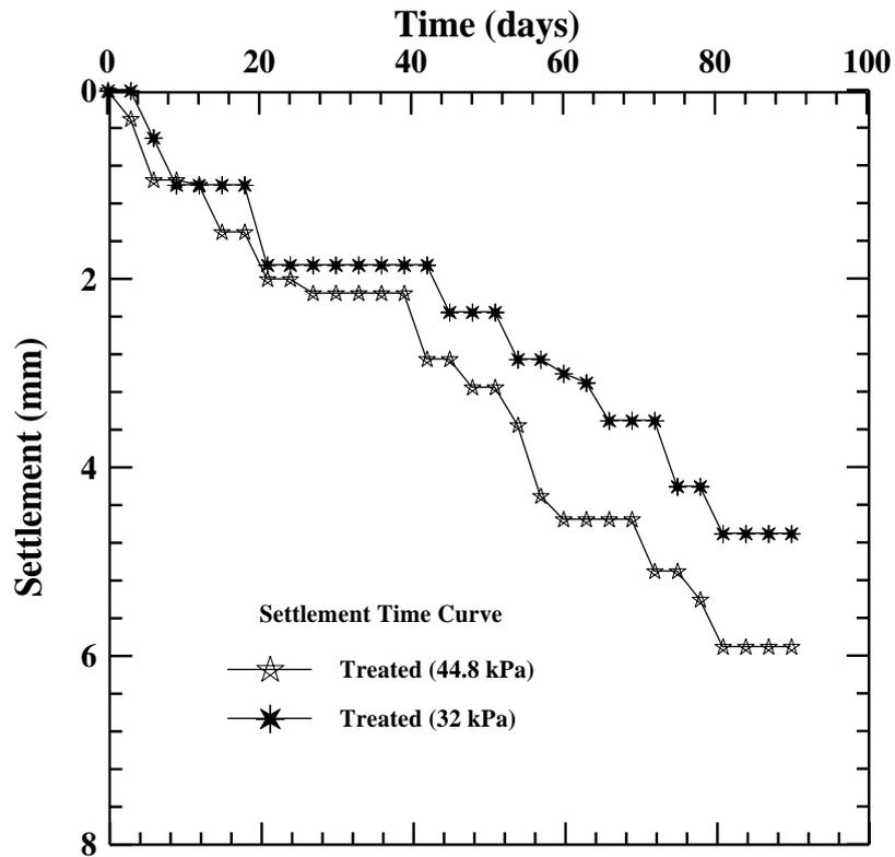
*Figure (5.24) Settlement versus Time (Effect of Applied Stress)*
