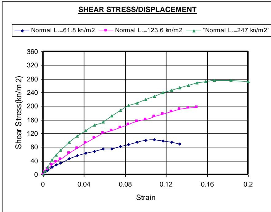
*Results of Direct Shear (Sample 3, Before Flooding)*
