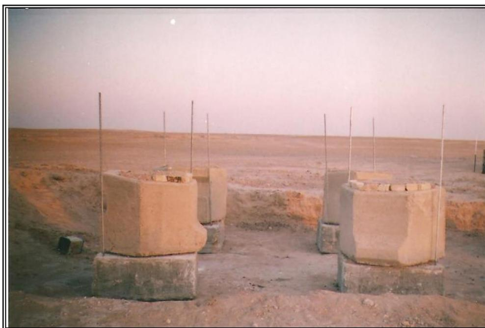
*Plate (4.9) The Footings under the Action of the First Stress Increment of 16 kPa*
