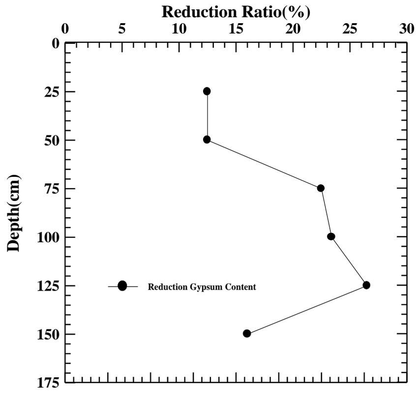
*Figure (5.14) Reduction in Gypsum Content with Depth*
