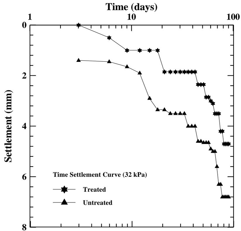
**Figure (5.29) Settlement versus Time (Semi log Scale)**
