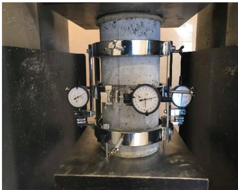
Figure 2: Modulus of elasticity test using compressometer.
