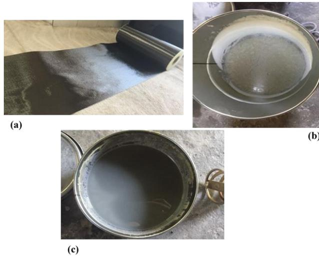
Figure 4: CFRP and epoxy resin: (a) CFRP roller; (b) epoxy resin component A; and (c) epoxy resin component B.
