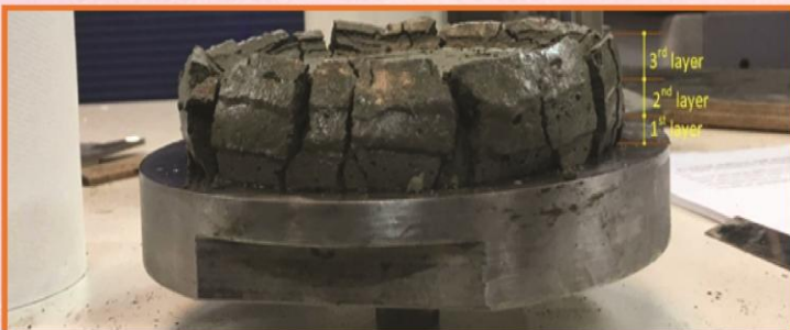
.Figure (5) Triple layers of the mortar after squeezing under a uniaxial compression load
