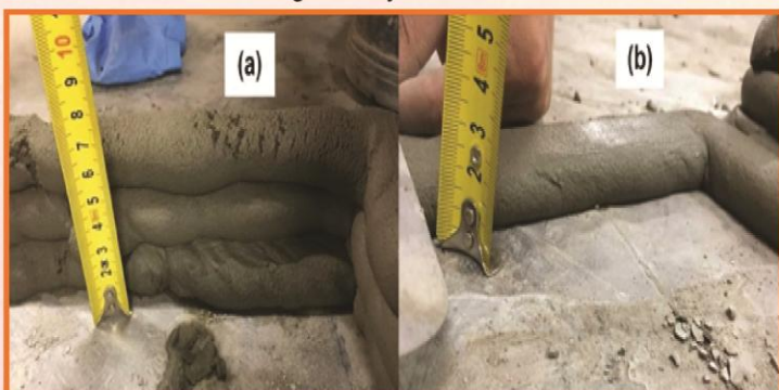
Figure (10) (a) Three layers of the printed object; (b) One layer of the printed object. For a printed object of over 120 mm (more than 7 layers), the oscillation at the arm of the robot increased in the end-tip of the arm which is most related to joint 4 and joint 6 in the robot [27].
