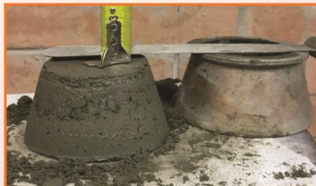
Figure (15) Mini-cone slump test for trial 8
