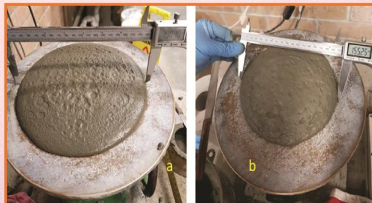
Figure (16) Spread-flow test: (a) for trial 5 which did not use fibre; (b) for the same trial by adding fibre with 1% polypropylene fibre
