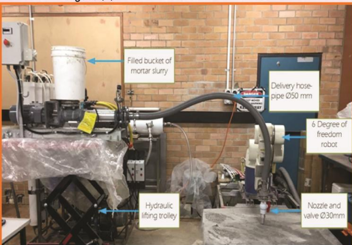
Figure (4) The final system with the progress cavity pump connected to the robot
