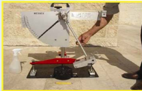
Figure 10 : Modified British Pendulum skid resistance tester
