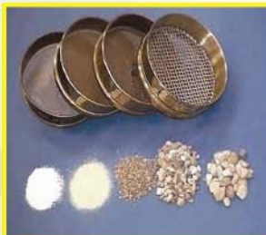
Figure 11 : The standard gradation and sieve analysis test
