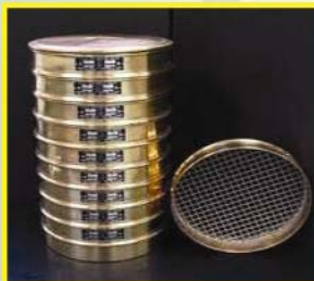
Figure 12 : Set of Sieves (Sieve Analysis of Fine and Coarse Aggregates)
