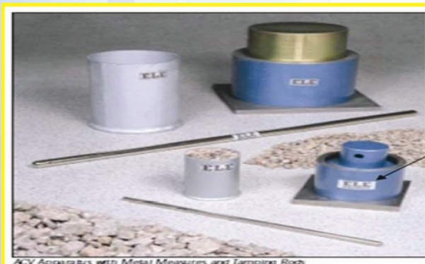
Figure 6 : Aggregate Crushing Value (ACV) and Ten Percent Fines Value (TFV) BS 812: 110, 111
