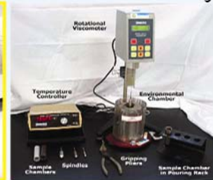
Figure 23: Major RV equipment into the sample chamber.
