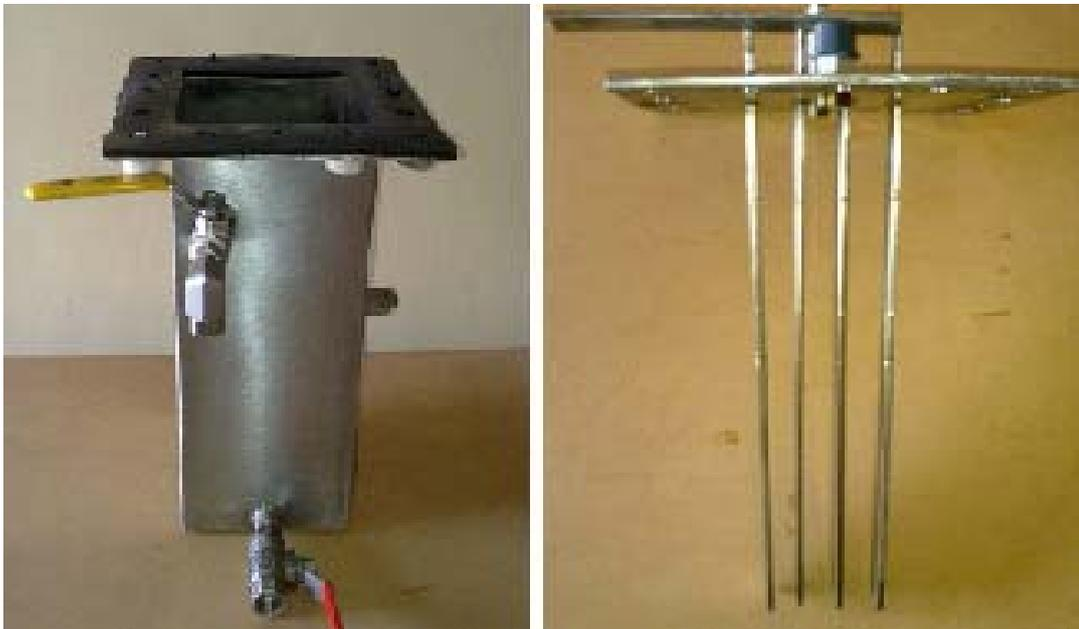
**Figure2.** Arrangements of electrodes in second design of electrolyser.
