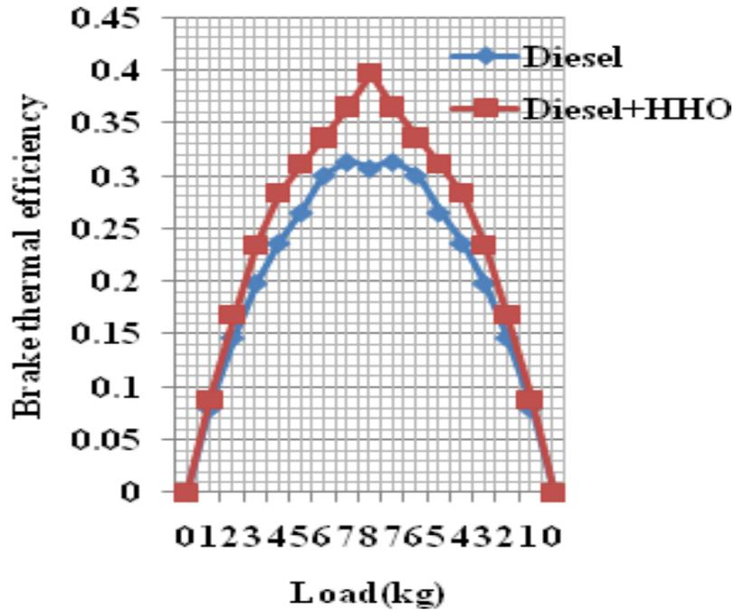
Figure 7. Graph of brake thermal efficiency in percent v/s load in kg.
