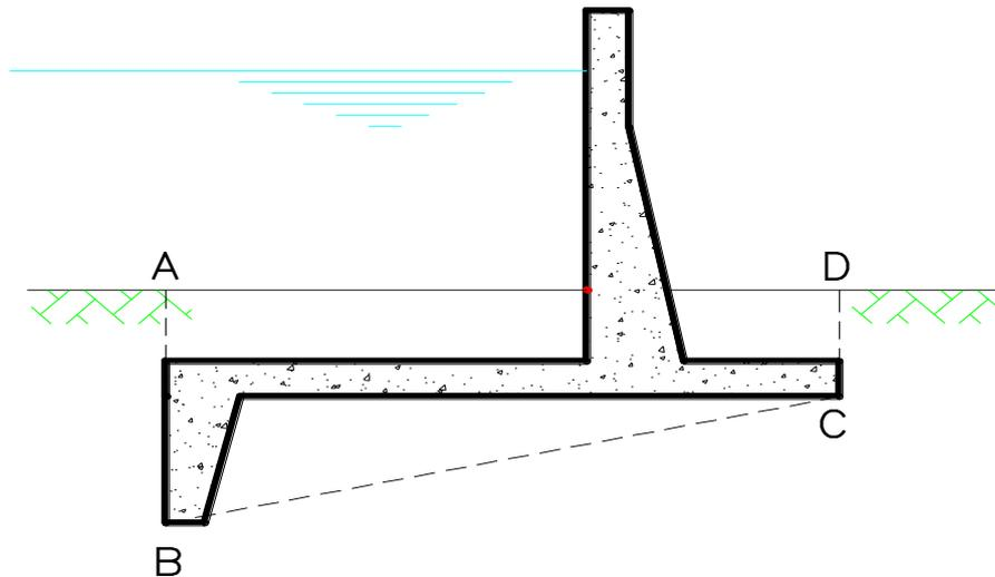
**Figure (6)** Seepage path for wall with upstream cutoff
