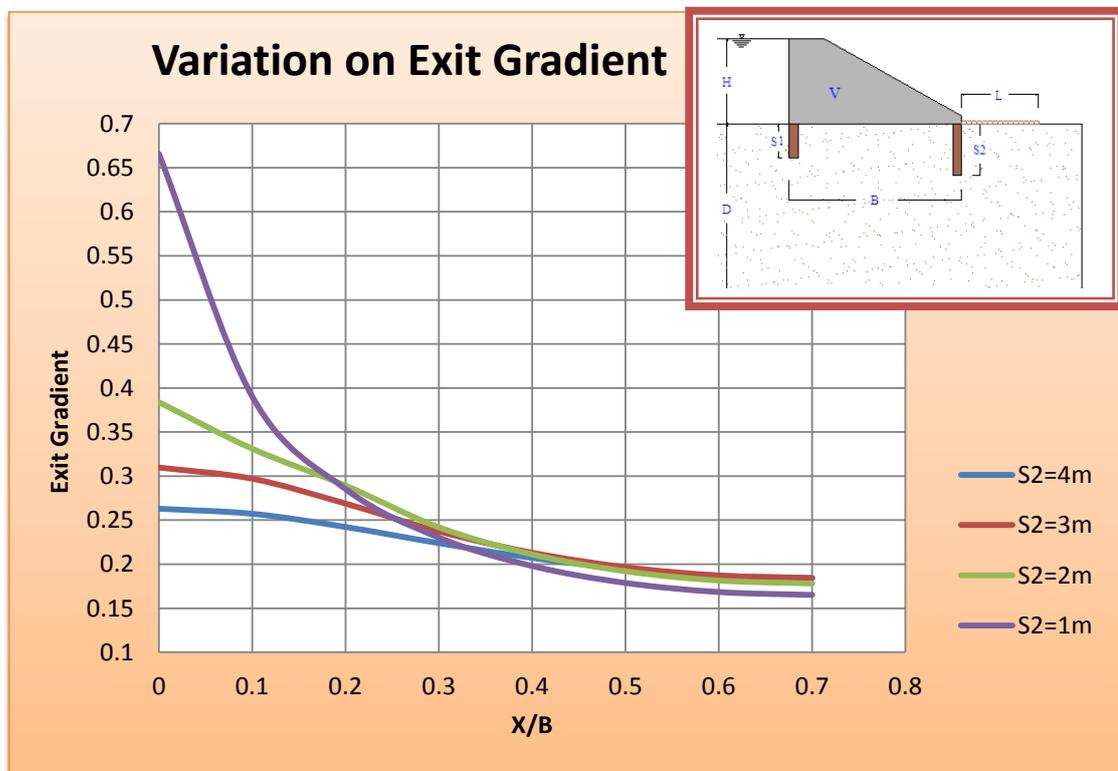
Fig (10) Variation of Exit Gradient for Hydraulic Structure with Downstream Cutoffs for  $S_1=3$ ms.
