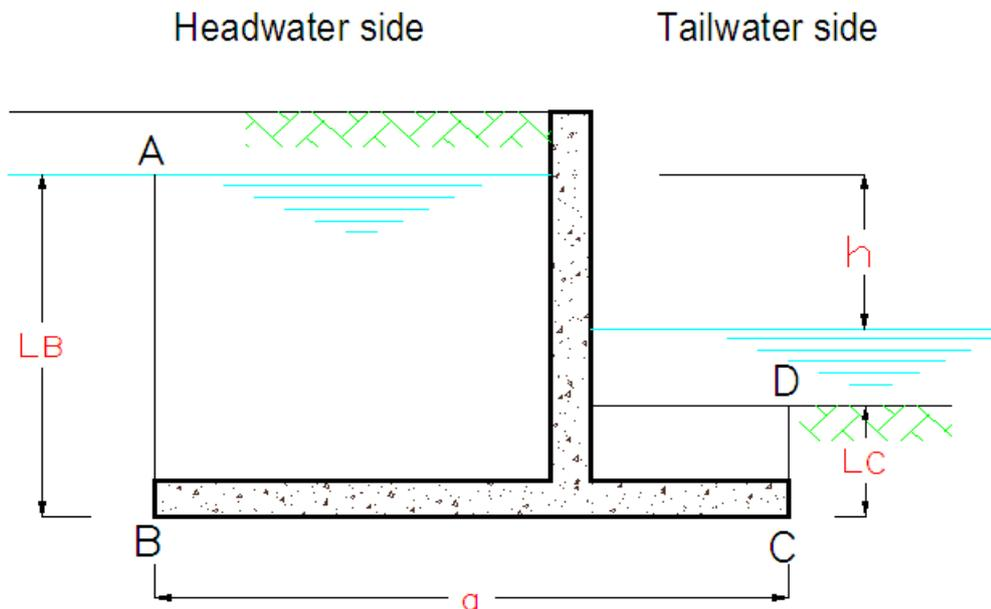
**Figure (5)** Line of seepage method for water pressures
