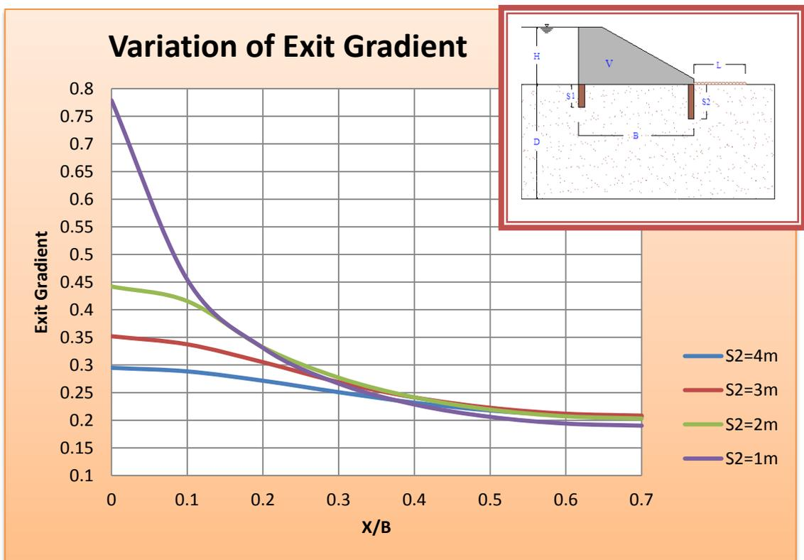
Fig (12) Variation of Exit Gradient for hydraulic structure with downstream cutoffs for  $S_1=1\text{ms}$ .
