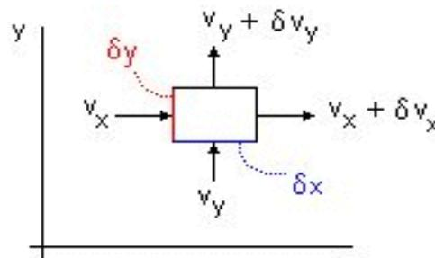
Figure (3) rectangular element with dimensions  $\delta x$ ,  $\delta y$  (Harr, 1962)
