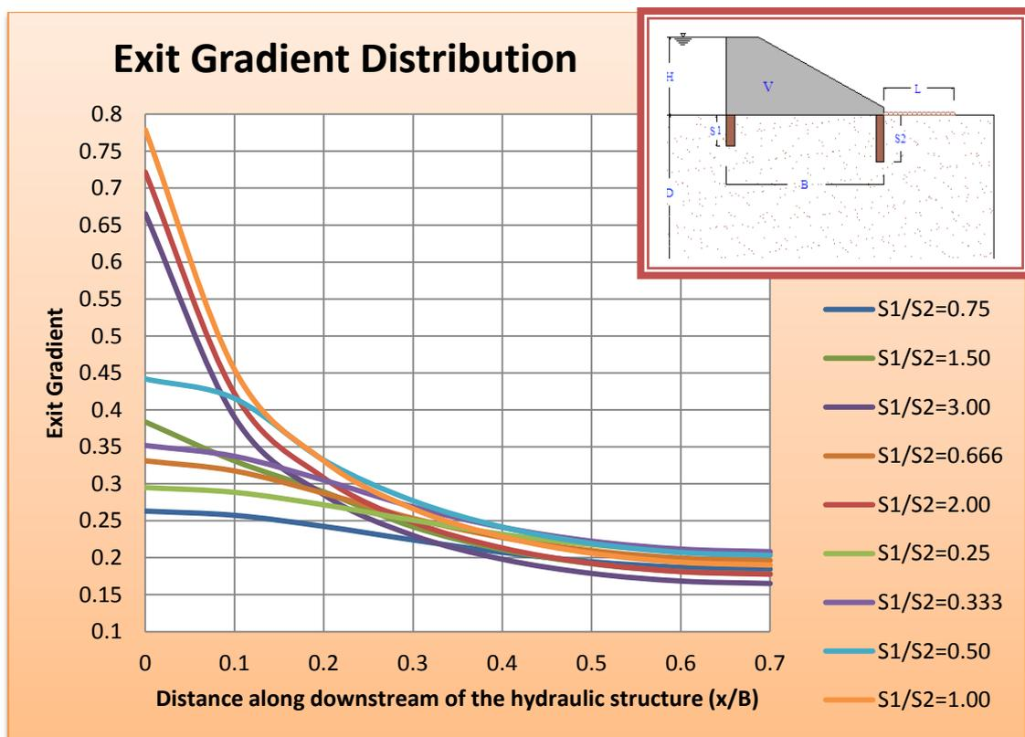
Fig (9) Exit Gradient Distribution under Hydraulic Structure with Different Depth of Upstream and Downstream Cutoffs for H= 5m and D=10m.
