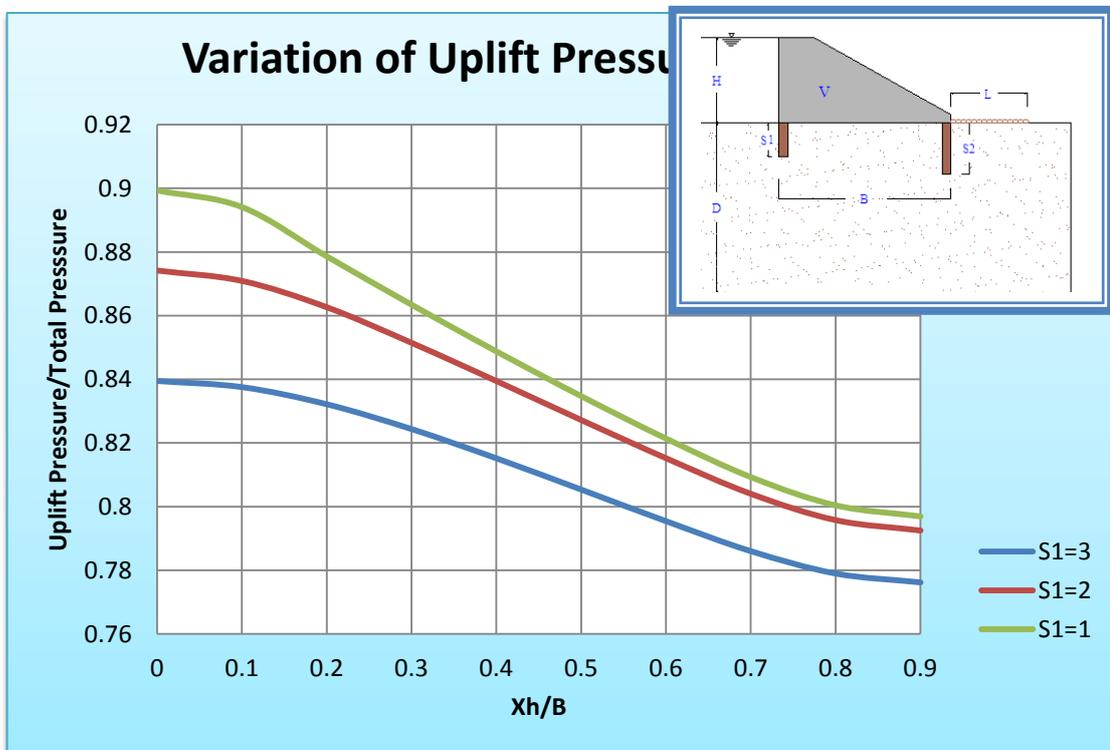
Fig (16) Variation of Uplift Pressure under a Hydraulic Structure Using Geo-Studio Results for  $S_2=2m$
