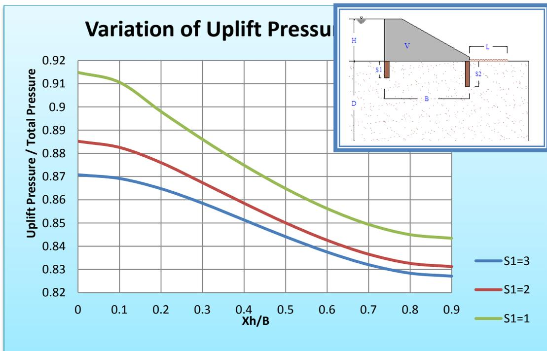
Fig (14) Variation of Uplift Pressure under a Hydraulic Structure Using Geo-Studio Results for  $S2=4m$ .
