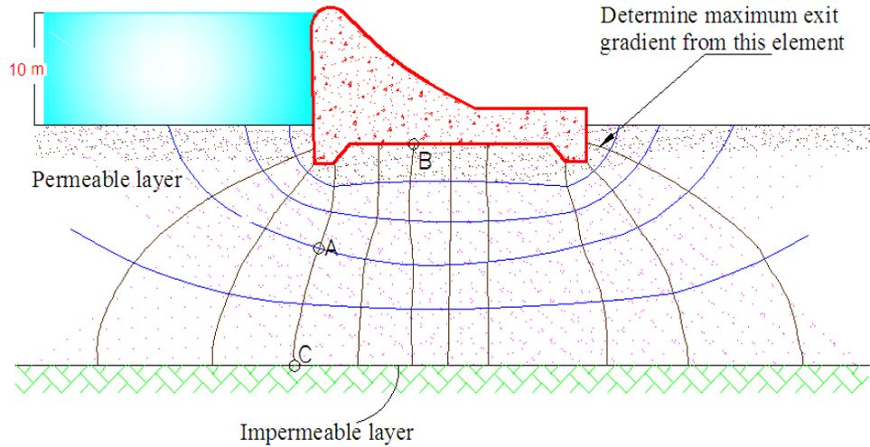
Figure (7) Flow net under a dam, (Harza ,1935)
