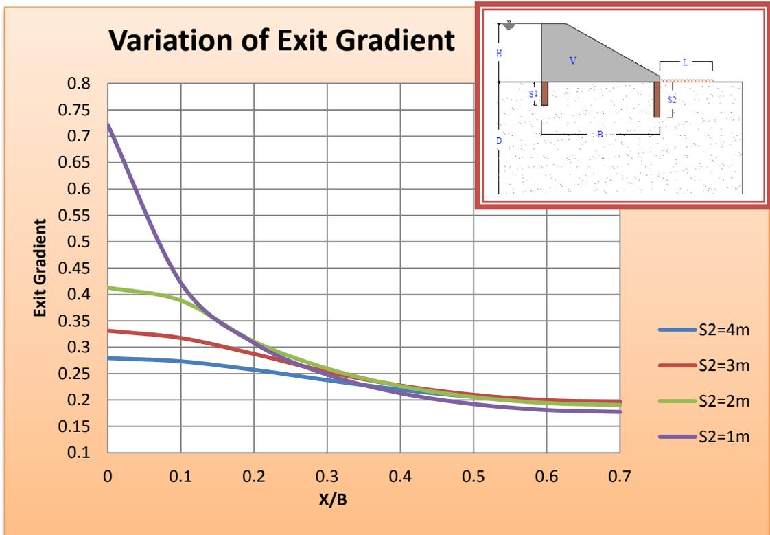
Fig (11) Variation of Exit Gradient for hydraulic structure with downstream cutoffs for  $S_1=2\text{ms}$ .
