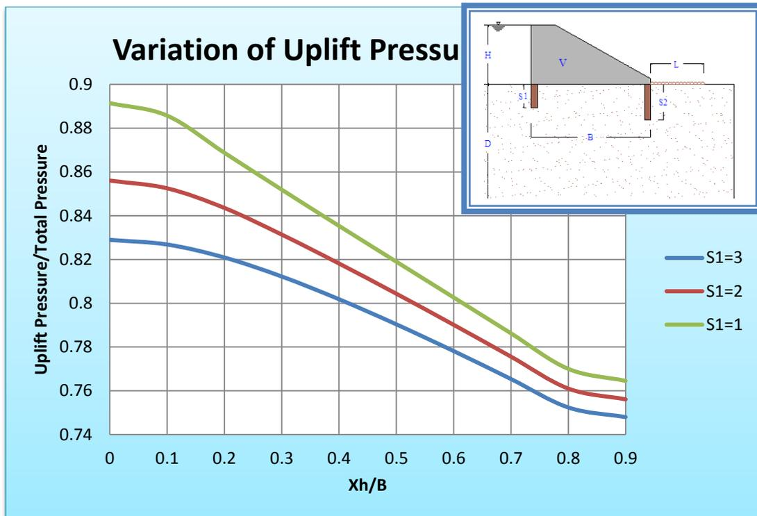
Fig (17) Variation of Uplift Pressure under a Hydraulic Structure Using Geo-Studio Results for S2=1m.
