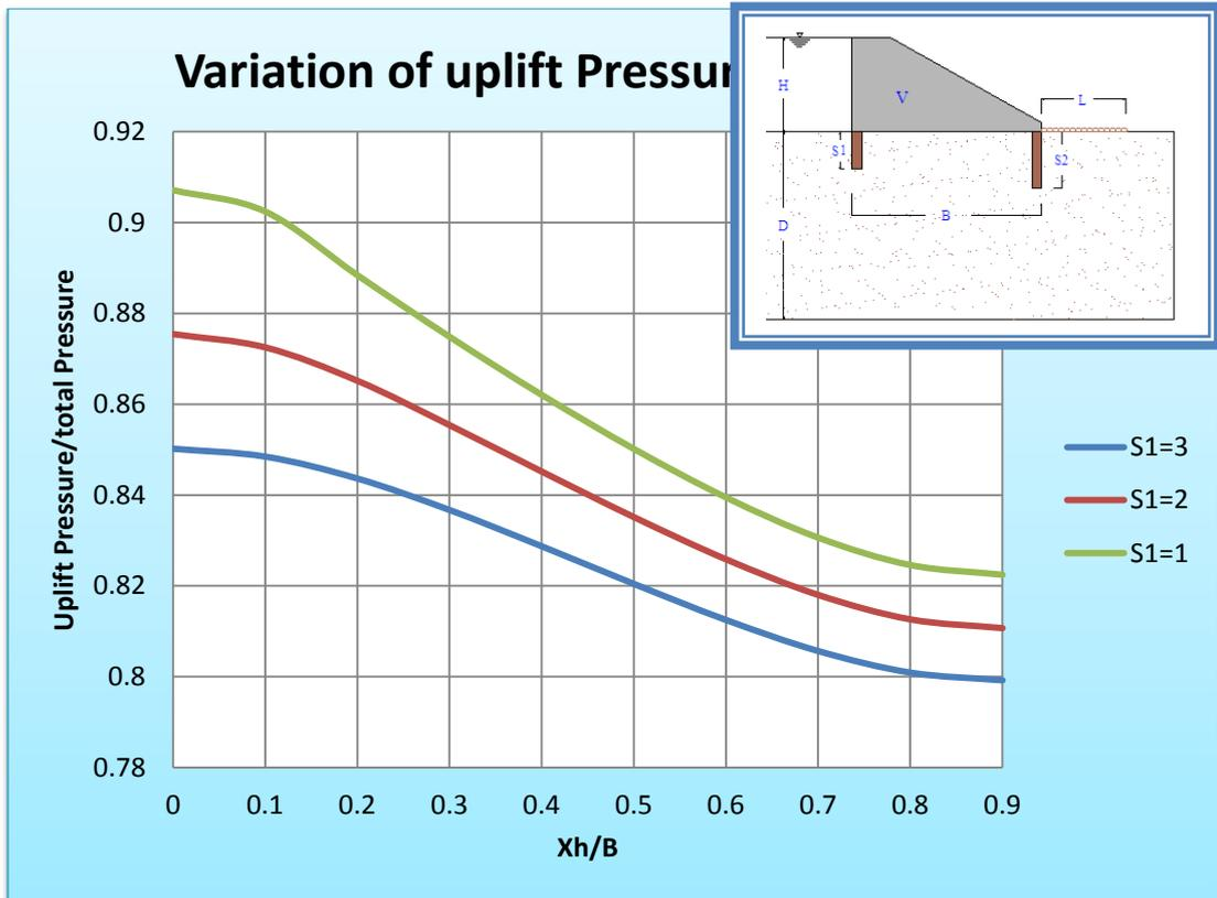
Fig (15) Variation of Uplift Pressure under a Hydraulic Structure Using Geo-Studio Results for  $S_2=3m$
