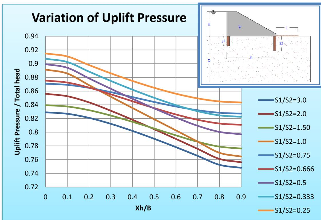
**Fig (13)** Variation of Uplift Head under a Hydraulic Structure Using Geo-Studio Model
