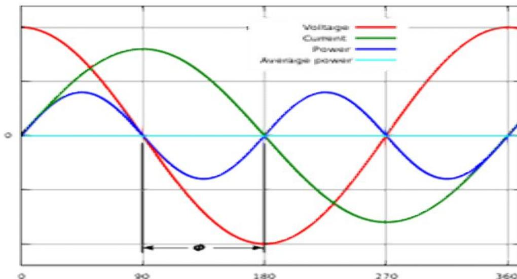
Instantaneous and average power calculated from AC voltage and current with a zero power factor ( $\varphi = 90$ ,  $\cos \varphi = 0$ ). The blue line shows all the power is stored temporarily in the load during the first quarter cycle and returned to the grid during the second quarter cycle, so no real power is consumed.
