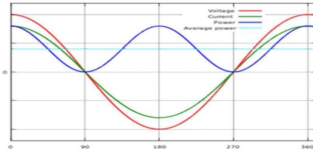
Instantaneous and average power calculated from AC voltage and current with a unity power factor ( $\varphi = 0$ ,  $\cos \varphi = 1$ ). Since the blue line is above the axis, all power is real power consumed by the load.
