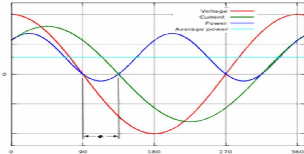
Instantaneous and average power calculated from AC voltage and current with a lagging power factor ( $\varphi = 45^\circ$ ,  $\cos \varphi = 0.71$ ). The blue line shows some of the power is returned to the grid during the part of the cycle labeled
