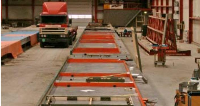
When collapses amenities such as electra tours/boxes, mounting pairing, slots, lifting facilities and window and door pairing, are placed, the first layer lightweight concrete.
