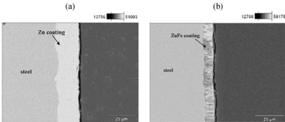
The galvanizing process not only prevents corrosion of various “soft” metals, but adds to the strength of the original, uncoated metal. Obviously, *galvanized metal* is thicker than uncoated metal, thus fittings and fastenings are generally measured with the additional galvanizing mil specs in mind. Various American Society for Testing and Materials (ASTM) specifications provide guidelines and continuity for the thickness of galvanized metals.
