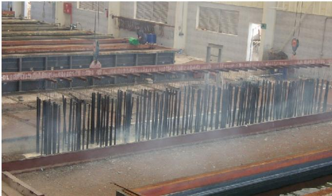
A process by which zinc is coated over corrosive metals is known as galvanizing. The galvanizing process is actually a method of coating corrosive metals, such as steel and iron, with a non-corrosive metal. Zinc is melted and applied, usually via what’s known as a hot dip, to the metal, providing a coating of corrosion protection from one mil to just over four mils thick. When cured, the zinc, through reaction with the coated metal, becomes zinc carbonate.
