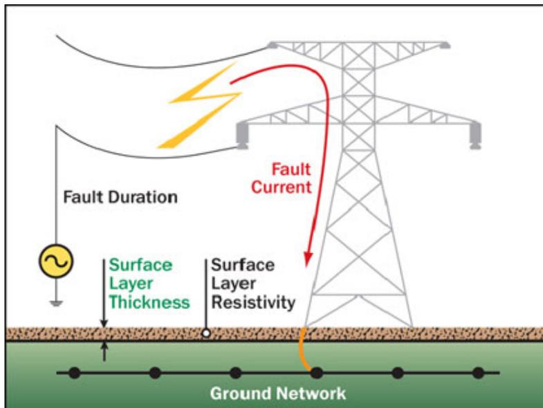
For example: Many utility companies require at a minimum that a simple ground ring be installed at least 18 inches below ground and 3 feet from the perimeter of all metal objects. This ground ring is also referred to as a counterpoise.
