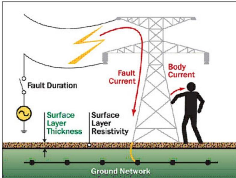
For example if a person happens to be touching a high-voltage tower leg when a fault occurs, the electricity would travel down the tower leg into the person’s hand and through vital organs of the body. It would then continue on its path and exit out through the feet and into the earth. Careful analysis is required to determine the acceptable Fibrillation Currents that can be withstood by the body if a fault were to occur.
