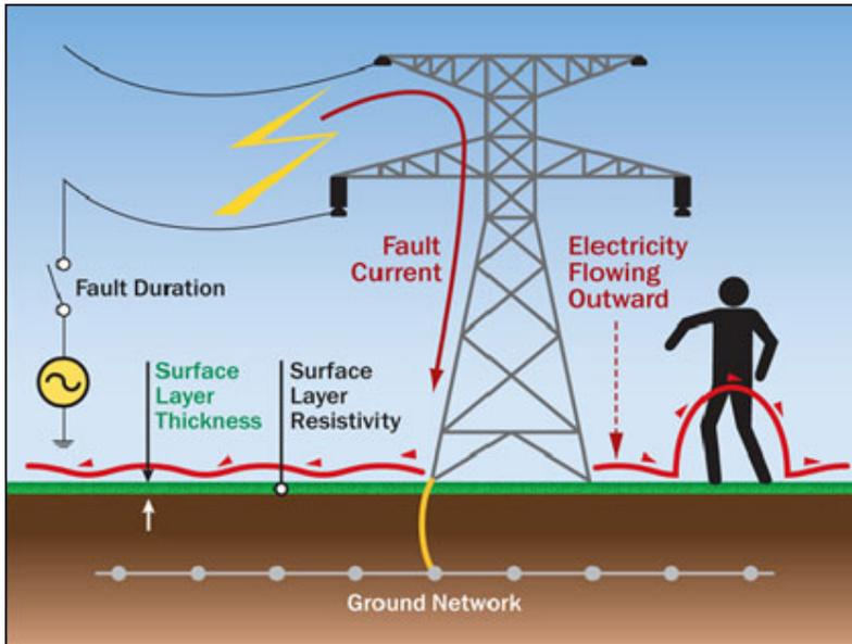
In the case of Step Potentials or step voltage, electricity will flow if a difference in potential exists between the two legs of a person. Calculations must be performed that determine how great the tolerable step potentials are and then compare those results to the step voltages expected to occur at the site.
