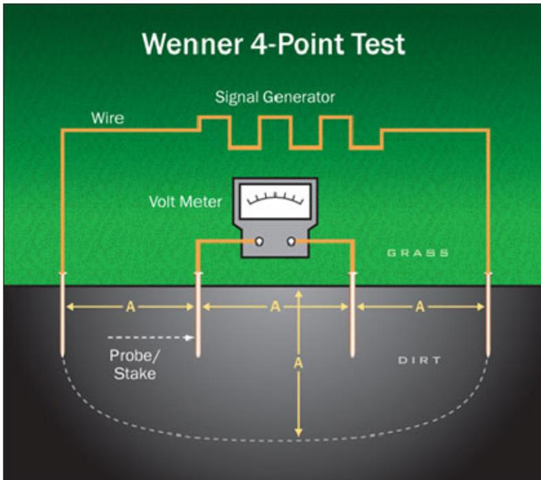
Electrical resistivity is the measurement of the specific resistance of a given material. It is expressed in ohm-meters and represents the resistance measured between two plates covering opposite sides of a 1 m cube. This soil resistivity test is commonly performed at raw land sites, during the design and planning of grounding systems specific to the tested site.
