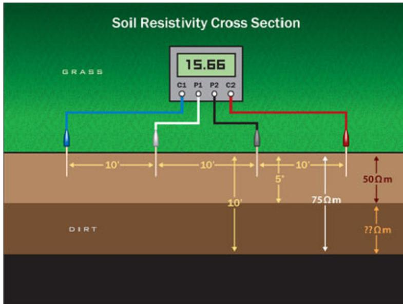
As you can see in the following diagram, if you have a 2' reading of 20 ohm-meters and a 10' reading of 50-ohmmeter soil, the actual soil resistivity from 2' to 10' might be 100 ohm-meters (the point here is to illustrate a concept: pre-computed curves or computer software are needed to properly interpret the data). The same follows true for larger pin spacings. The shallowest readings are used over and over again in determining the actual resistivity at depth.
