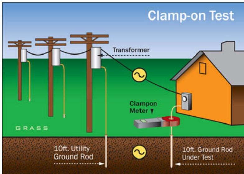
Understanding the proper field application of this test is vital to obtaining accurate results. The induced frequency test can test grounding systems that are in use and does not require the interruption of service to take measurements.
