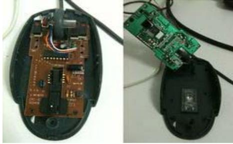
A PCB in a computer mouse. The Component Side (left) and the printed side (right).
