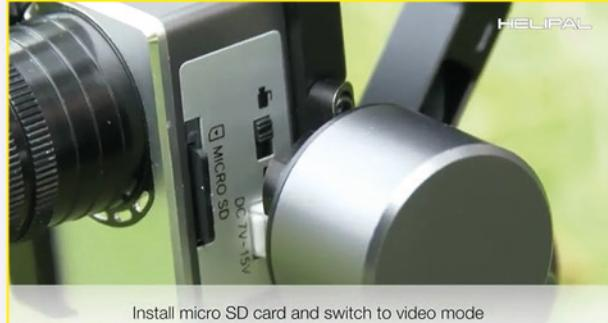
Install micro SD card and switch to video mode
