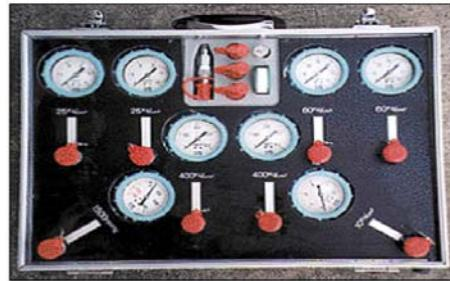
Complete set of hydraulic pressure measuring instrument and devices
